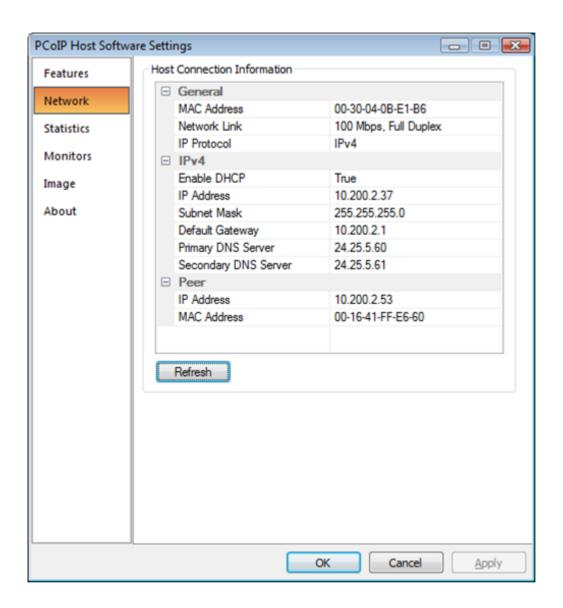
The *Network* tab shows the current network information for the host. This tab also reports status information on the NIC of the PCoIP host (speed, duplex setting, and link state – up/down). It also displays the IP and MAC addresses of the client connected to the host under the Peer settings.
